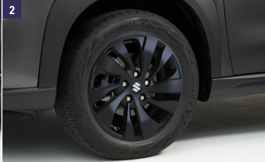
2 | Alloy Wheel “17” 1 WVTA EU Gloss Black painted version of OE painted wheel for GL and GL+ grade, 6.5 J x 17” suitable for 215/55R17 tires, centre cap is not included. Part No. 43210-64RF0-0CE G I J K
