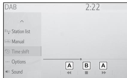
**A** Select to jump forward/backward by 10 seconds. Select and hold to fast forward/backward.
