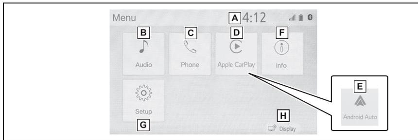
**A** Displays the clock. Select to display the clock settings screen. (→P.49)
