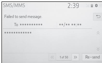
"Re-send": Select to re-send the message. This switch is displayed if sending the text message has failed.
