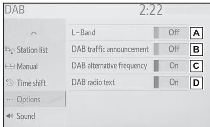
**A** Select on/off to set L-band in the tune range. When “Off” is selected, the physical channel range for tuning operations is limited to Band III, excluding for preset operations. When “On” is selected, the physical channel range for tuning operations includes Band III and L-band.
