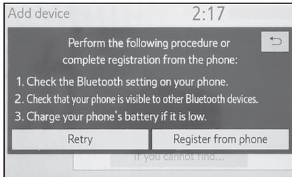
3 Check that the following screen is displayed, and register the Bluetooth® device using your Bluetooth® device.
