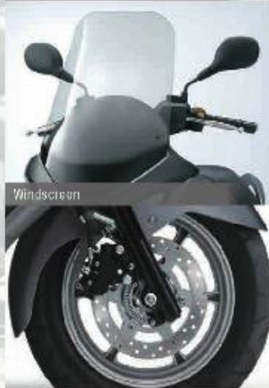
Front & rear disc brakes, optional ABS
